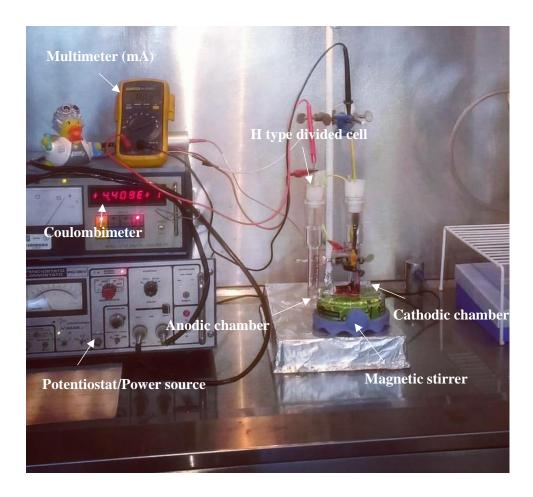
Figure S1. Electrolysis setup for the thiocarbonates reduction in hydroalcoholic media.
