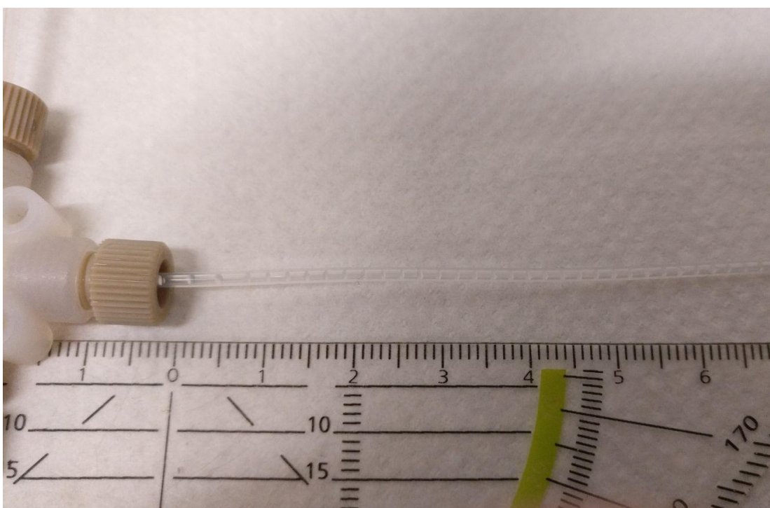
Figure S11: Image of the segmented flow at an oxygen : liquid ratio of three to one at the beginning of the reactor.
