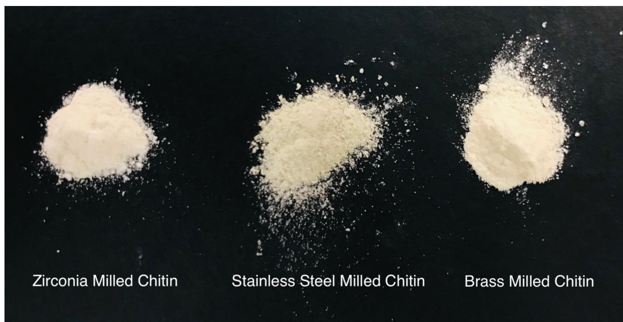
Figure S5: Chitin samples from left to right, chitin milled in zirconia, chitin milled in stainless steel jar and ball (30 min, 29.5 Hz), chitin milled in brass jar and ball (30 min, 29.5 Hz).
