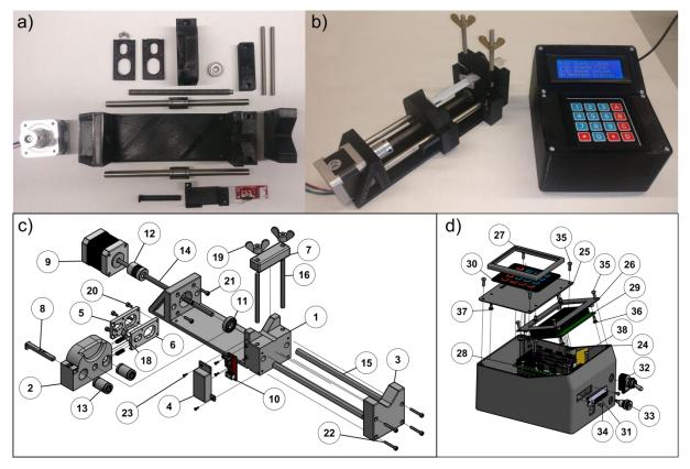
**Figure S2:** a) Unassembled parts used for one syringe pump. b) Assembled syringe pump and controller c) Exploded-view CAD drawings of the pump. d) The controller.
