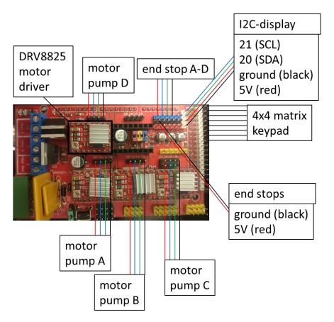
Figure S3: Wiring diagram of the syringe pump rack.
