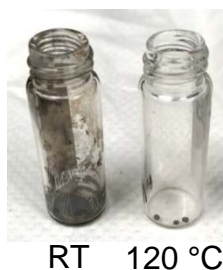
Figure S1: Silver mirroring is not observed at high temperature.
