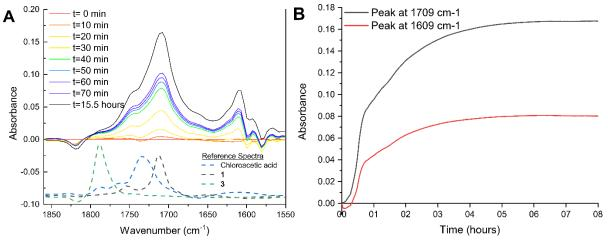
**Figure S5:** In situ IR spectroscopy measurement of the reaction. A: difference spectra in time relative to t = 0 and measured reference spectra of isolated compounds (offset vertically). B: Kinetic profile of the reaction based on peak height as a function of time.
