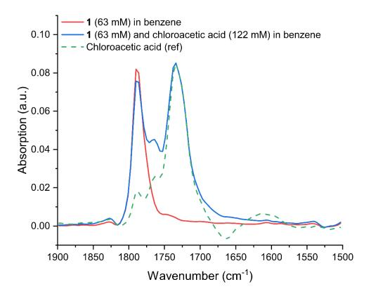
**Figure S8:** FTIR spectra. Red: IR spectrum of **1** in benzene. Blue: IR spectrum of the mixture from the red spectrum after addition of chloroacetic acid. Dashed green: IR reference spectrum of chloroacetic acid.
