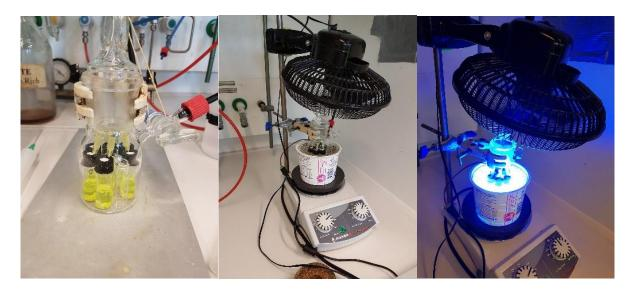
**Figure S3:** The glass jar with Schenk connection and the setup used for photocatalytic batch reaction.
