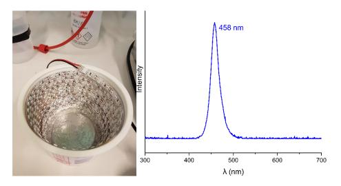
Figure S1: Top view and emission spectra of the 458 nm LED source.
