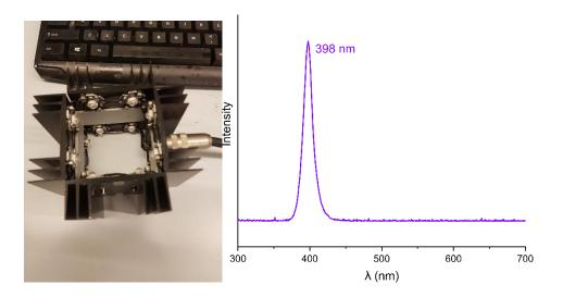
Figure S2: Top view and emission spectra of the 398 nm LED source.
