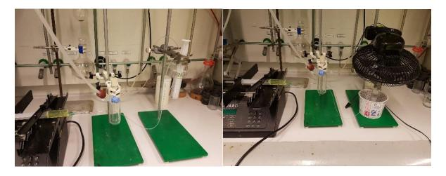
Figure S4: The setup used for photocatalysis in flow.
