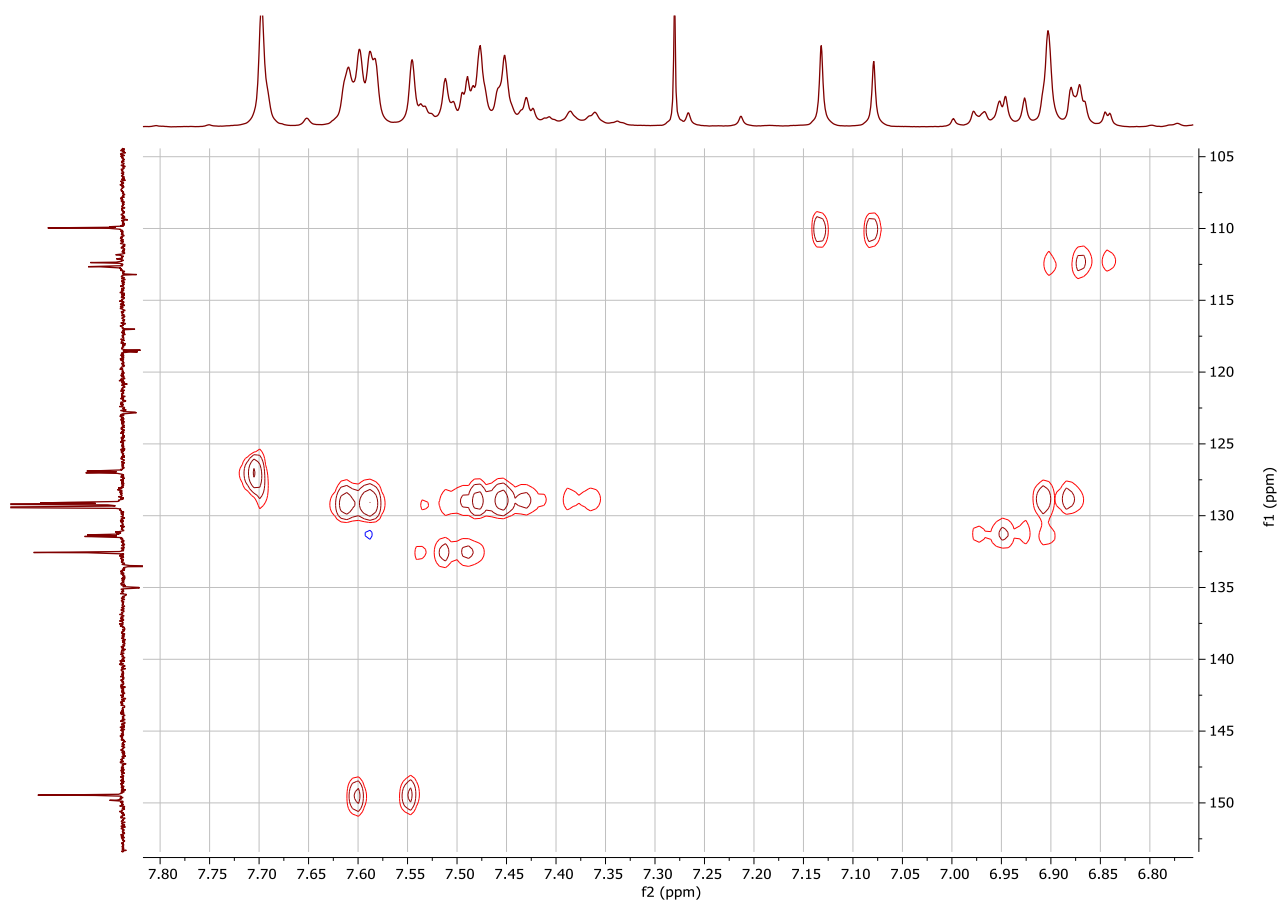
^1\text{H} - ^{13}\text{C} HSQC NMR spectrum of 3a
