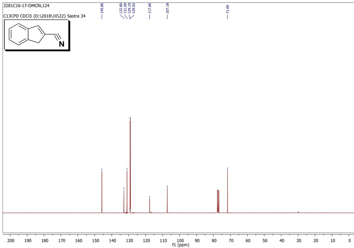
**Fig. S4**  $^{13}\text{C}$  NMR spectrum *1H*-indene-2-carbonitrile (**6b**).
