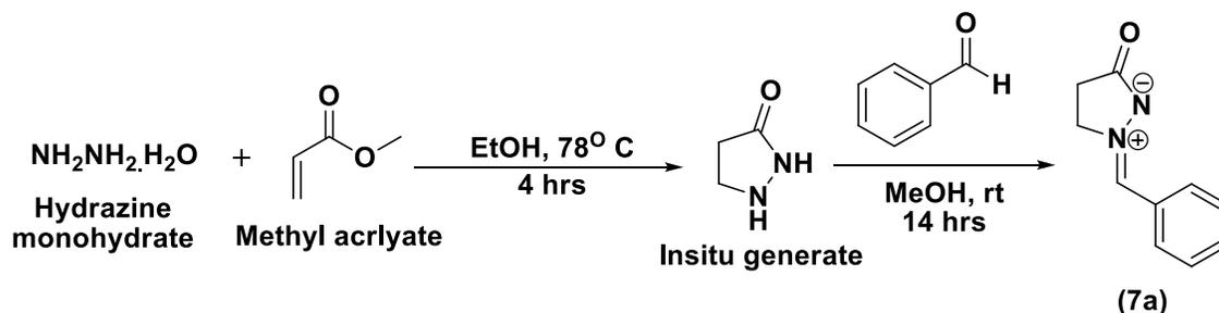
**Scheme. 1** Synthesis of 1-Benzylidene-3-oxopyrazolidin-1-ium-2-ide (7a).
