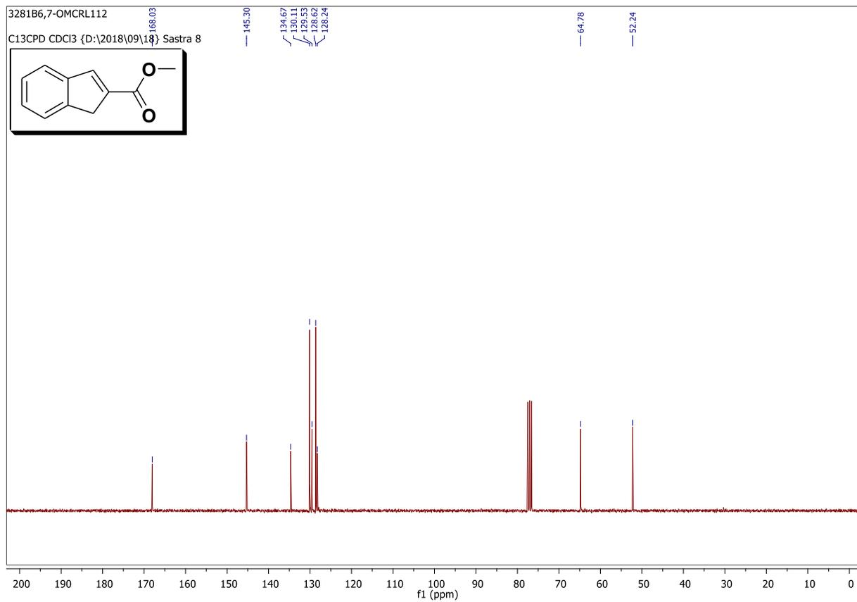
Fig. S2  $^{13}\text{C}$  NMR spectrum of methyl 1*H*-indene-2-carboxylate (**6a**).
