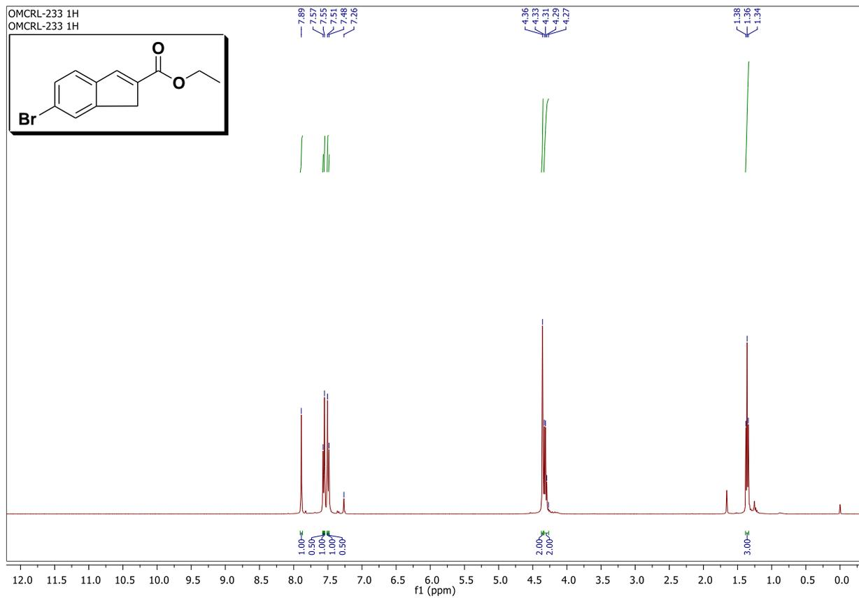
**Fig. S11**  $^1\text{H}$  NMR spectrum of ethyl 6-bromo-1H-indene-2-carboxylate (**6f**).
