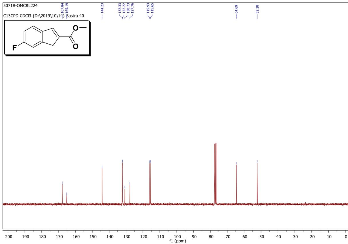
Fig. S20 <sup>13</sup>C NMR spectrum of methyl 6-fluoro-1*H*-indene-2-carboxylate (**6j**).
