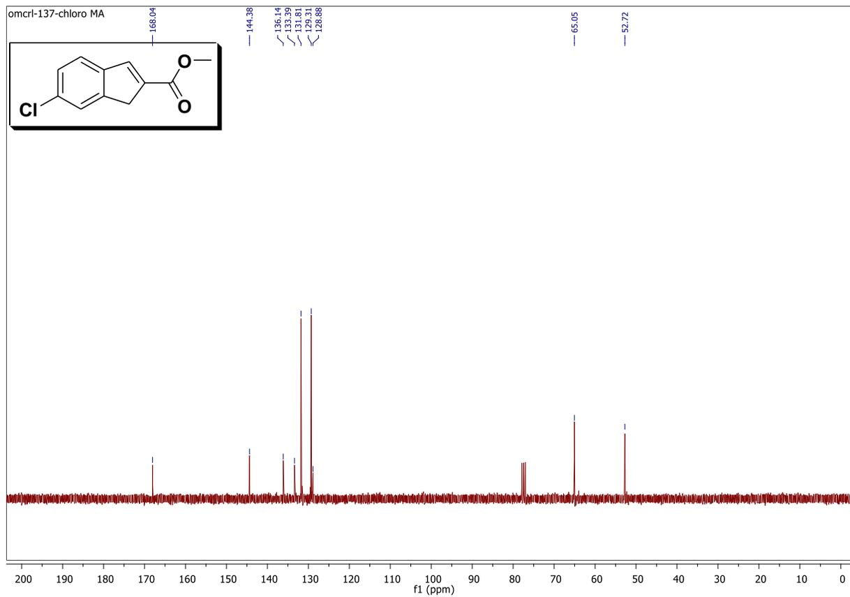
Fig. S14 <sup>13</sup>C NMR spectrum of methyl 6-chloro-1*H*-indene-2-carboxylate (**6g**).
