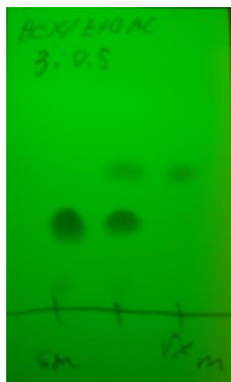
Figure S2. TLC for testing if -(\text{CH}_2)_2\text{Ph}(4\text{-OMe}) group can be deprotected using KHMDS. Left lane: \text{MeO}(\text{CH}_2)_2\text{Ph}(4\text{-OMe}) ( 3b ); middle lane: co-spot of materials on the left and right lanes; right lane: reaction mixture. Eluent: hexanes/EtOAc 3:0.5. The TLC indicates that 3b was consumed.
