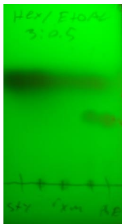
Figure S1. TLC for testing if -(\text{CH}_2)_2\text{Ph} group can be deprotected using KHMDS. Left lane: styrene; middle lane: reaction mixture; right lane: \text{Ph}(\text{CH}_2)_2\text{OMe} ( 3a ); 2 nd and 4 th lanes: co-spot of materials spotted on their adjacent lanes. Eluent: hexanes/EtOAc 3:0.5. The TLC indicates that 3a was consumed and styrene was formed.
