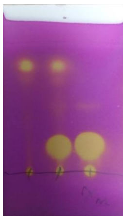
Figure S12. TLC for testing if -\text{CH}_2\text{C}\equiv\text{CMe} group can be deprotected by KHMDS. Left lane: \text{EtOCH}_2\text{C}\equiv\text{CMe} ( 3l ); middle lane: co-spot of materials on left and right lanes; right lane: reaction mixture. Eluent: hexanes/EtOAc 5:1. The TLC indicates that 3l was consumed.
