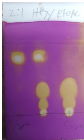
Figure S5. TLC for testing if the 2-(furan-2-yl)ethyl group can be deprotected by KHMDS. Left lane: 2-(2-methoxyethyl)furan ( 3e ); middle lane: co-spot of materials on left and right lanes; right lane: reaction mixture. Eluent: hexanes/EtOAc 2:1. The TLC indicates that 3e was consumed.
