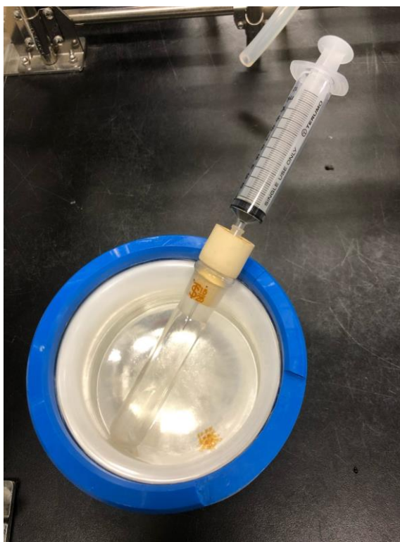
Figure S1. Addition of HCF 3 by a syringe
