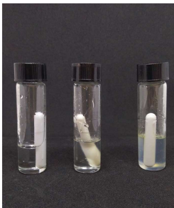
Figure 1 – From left, a vial with 2.5g of freshly prepared DES, a vial with DES used in two runs and a vial with DES used in four runs
