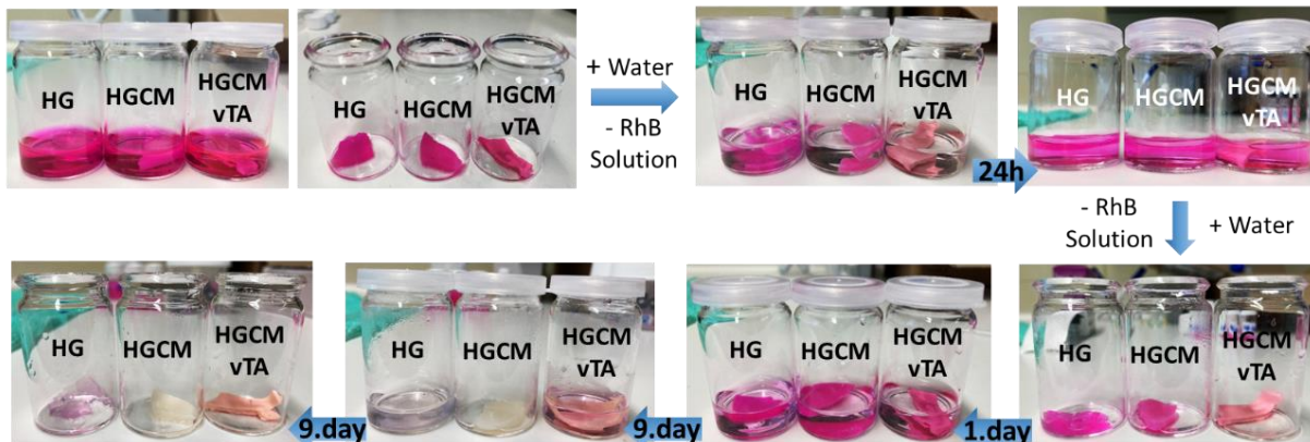
Figure S3: RhB dye releasing progress of HG, HGCM and HGCM-vTA at specified time intervals followed by UV-vis spectroscopy.
