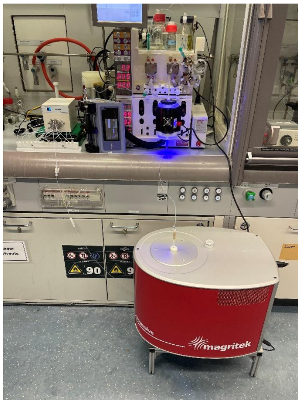
Figure S1: Experimental setup used for the flow experiments. The immobilised photoreactor module (in black) is connected to the bay 3 of the VapourtecR4, the blue halo is the marginal stray light escaping from the light filters at the top and bottom of the column holder. The syringe pump in purple is used to pump the reaction mixture, that is routed to the R4 pressure sensor, photoreactor module before flowing through the flow cell of the NMR and reaching the multi-position valve (in white, on the left) where the reactor outlet is fractionated into different vials for collection.
