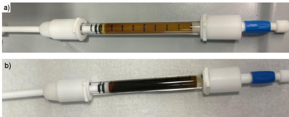
Figure S4: Photos of the packed column (a) before reaction (b) after irradiation at 70 °C for 12 hours.
