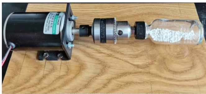
Figure S2: Self-made ball mill.
