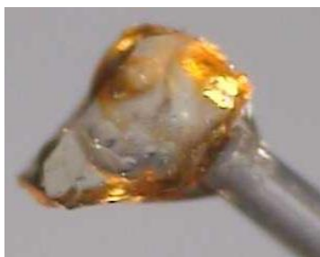
Figure S2. Specimen employed in the X-ray experiment. Real dimensions: 0.500 \times 0.350 \times 0.175 mm
