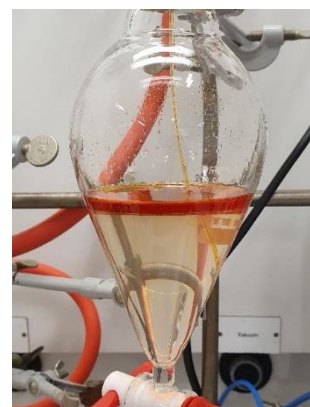
Figure S1: Collection of reactor output in a separatory funnel filled with brine.
