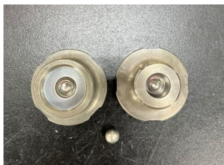
Figure S2. Stainless steel jar (1.5 mL) and ball (5 mm) used in this study.
