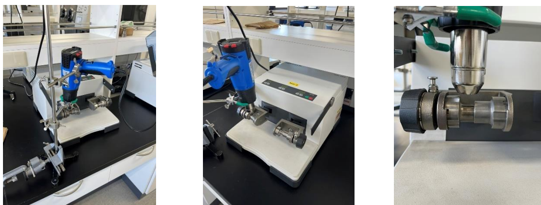
Figure S4. The set-up procedure for a heat gun on MM400.
