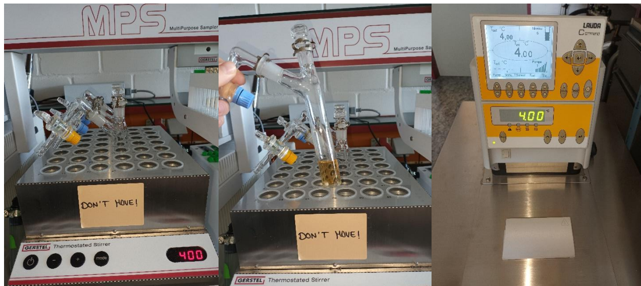
Figure S4: Michael addition (used for compounds S-17 and R-17 ). The Michael addition was performed in a self-made tube (shown in the middle). The similar to a Schlenk reaction vessel fitted into the LAUDA Proline RP855 refrigerated thermostat, which was able to hold the temperature at a constant temperature of 4 °C for at least 36 h. Photo by A. Ladwig, not used previously elsewhere.
