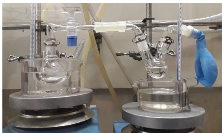
Figure S5: Cracking of paraformaldehyde (left flask) into formaldehyde. The left flask contains solid paraformaldehyde, which is thermally splitted. The formaldehyde produced is transferred into the solution of the right flask via the connection between tube and inlet. The balloon serves as monitor for the formaldehyde gas production. Photo by A. Ladwig, not used previously elsewhere.
