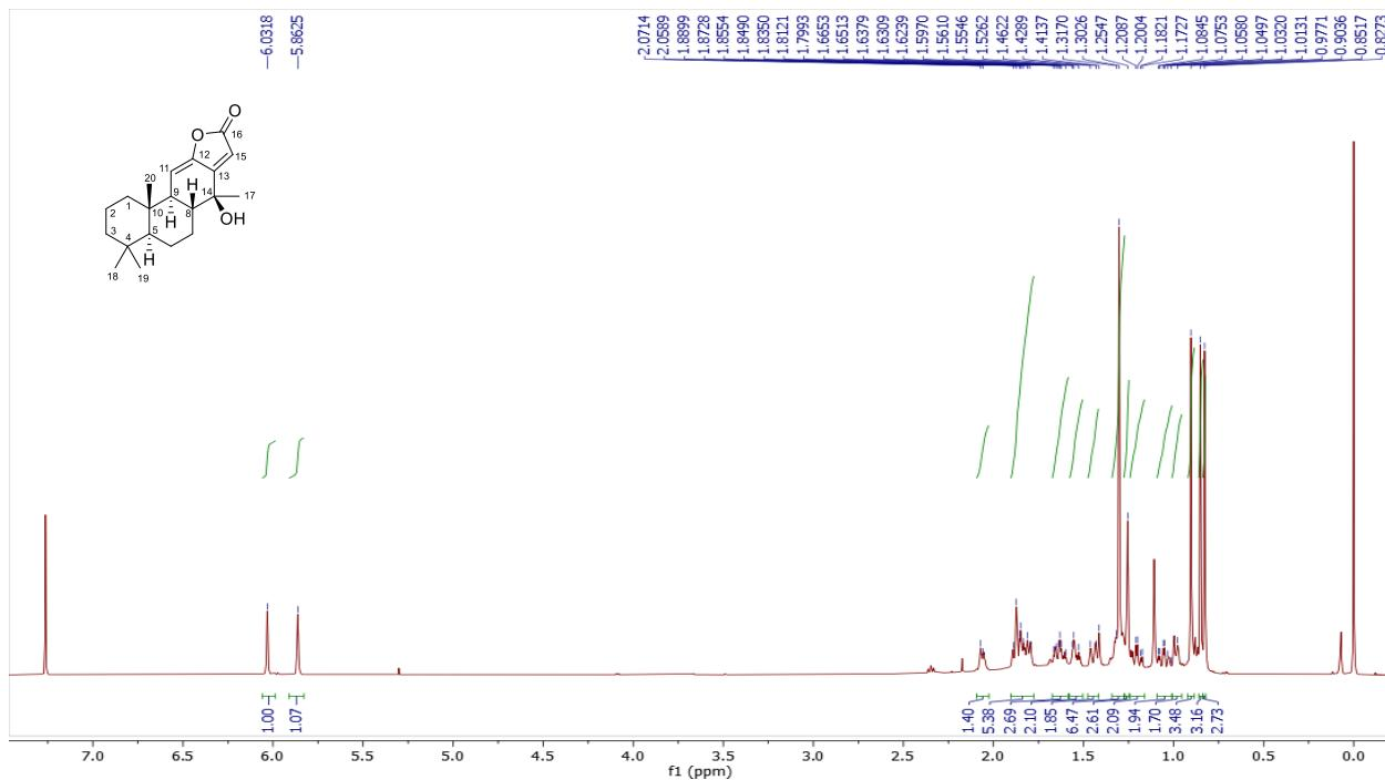
**Figure S1.**  $^1\text{H}$  NMR (500 MHz,  $\text{CDCl}_3$ ) spectrum of  $14\beta$ -hydroxycassa-11(12),13(15)-dien-12,16-olide (**1**).
