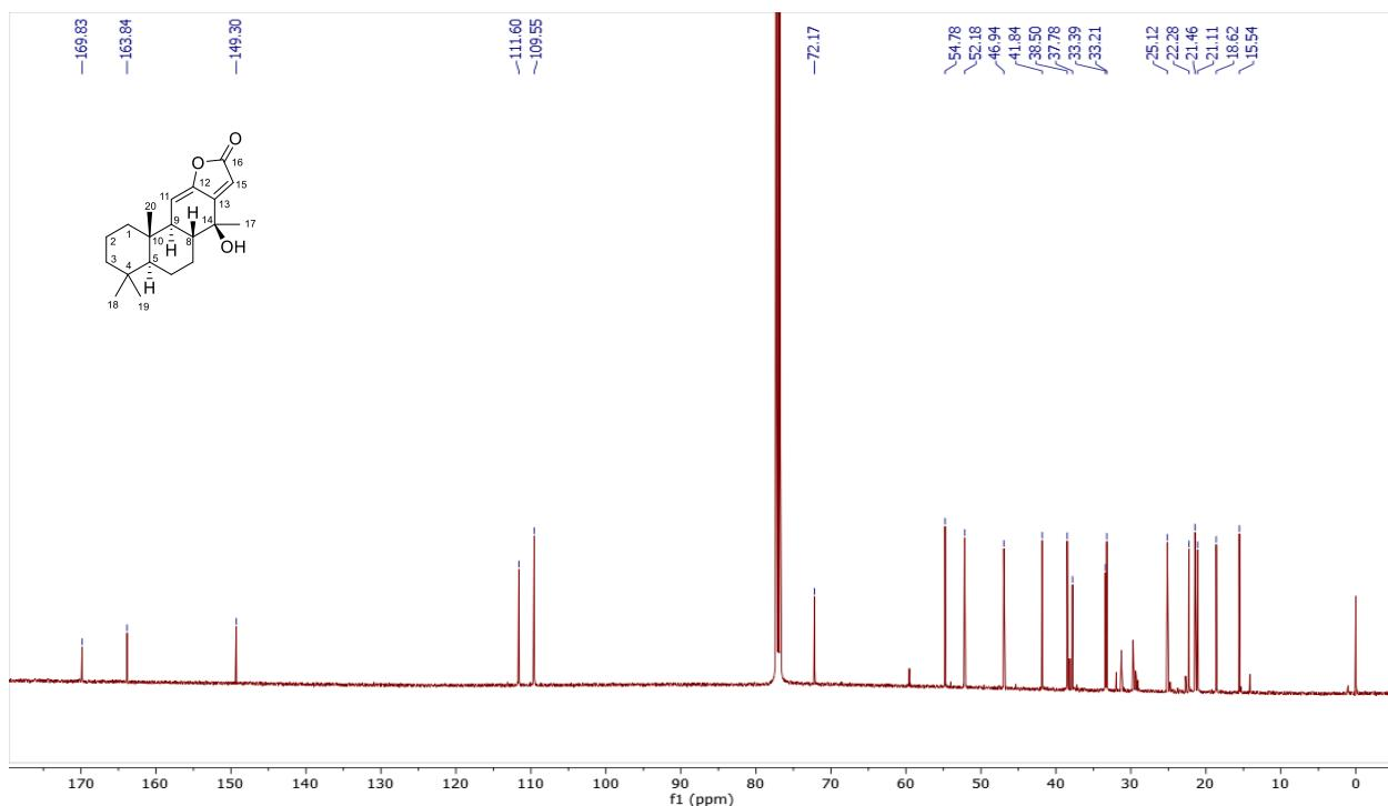
**Figure S2.**  $^{13}\text{C}$  NMR (125 MHz,  $\text{CDCl}_3$ ) spectrum of  $14\beta$ -hydroxycassa-11(12),13(15)-dien-12,16-olide (**1**).
