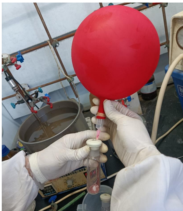
Figure S3: Bubbling from a \text{SO}_2\text{F}_2 balloon, or extracting and exchanging air for three times.
