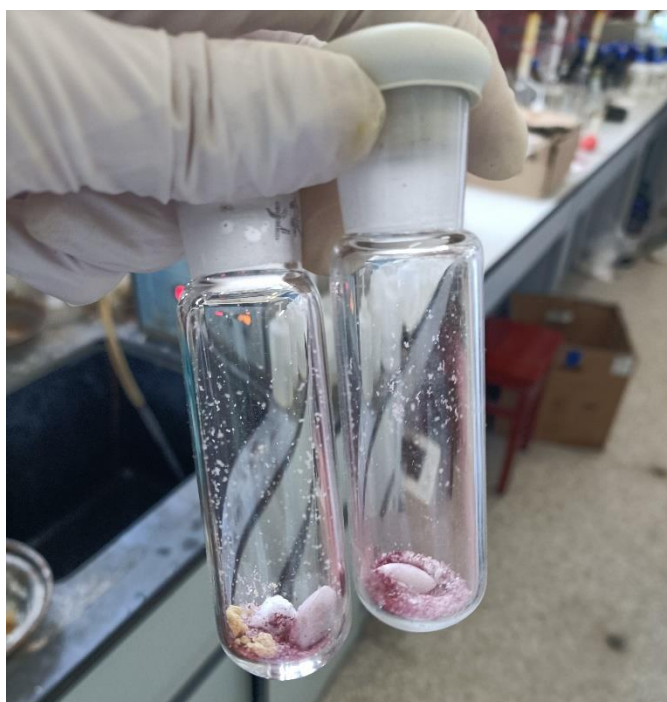
Figure S1: First, add all solid materials into an oven-dried tube or flask
