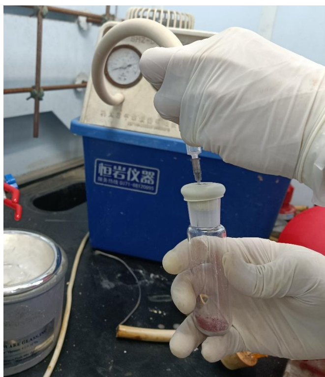
Figure S2: Using a vacuum pump to remove air
