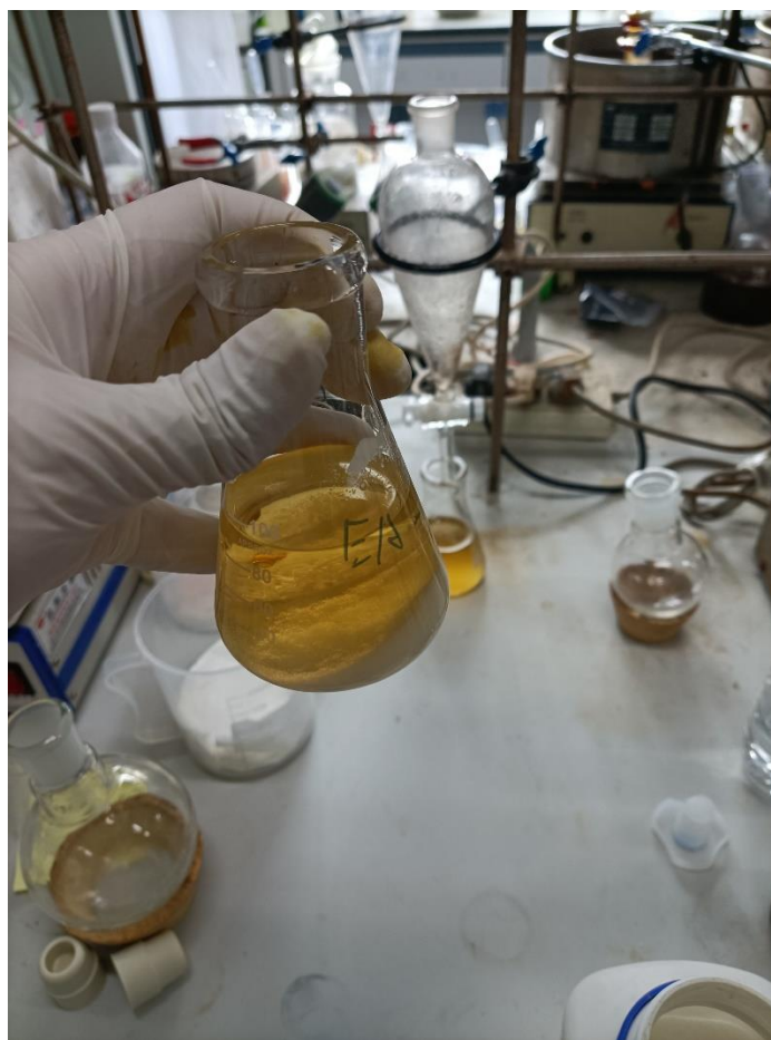
Figure S6: After the reaction is finished, extract with EA/water, take the EA layer and dry with anhydrous \text{Na}_2\text{SO}_4 .
