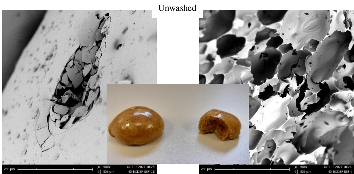
Figure S2. SEM of \beta -csp matrix unwashed showing outer (left) and inner(right) micrographs.
