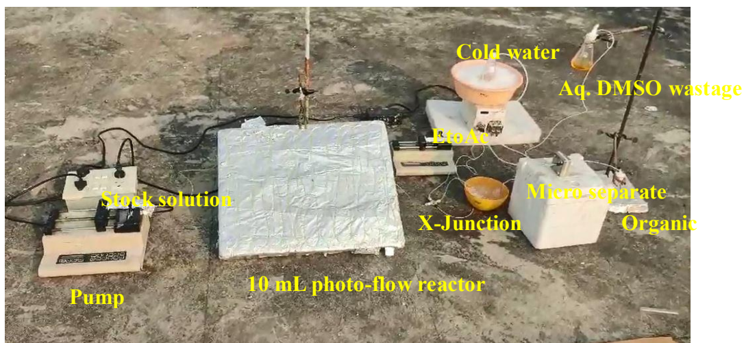
Figure S5. (a) Schematic graphic presentation of an integrated photo-flow Achmatowicz reaction, extraction, phase separation in continues flow manner. (b) Real image of an integrated photo-flow Achmatowicz reaction, extraction, phase separation set up.
