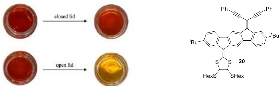
Figure S2: Visual experiment of compound 20 dissolved in CH 2 Cl 2 in two vials, one with closed lid (top) and one with open lid (bottom), to observe the impact of the presence of oxygen. The solutions were not shielded from light.
