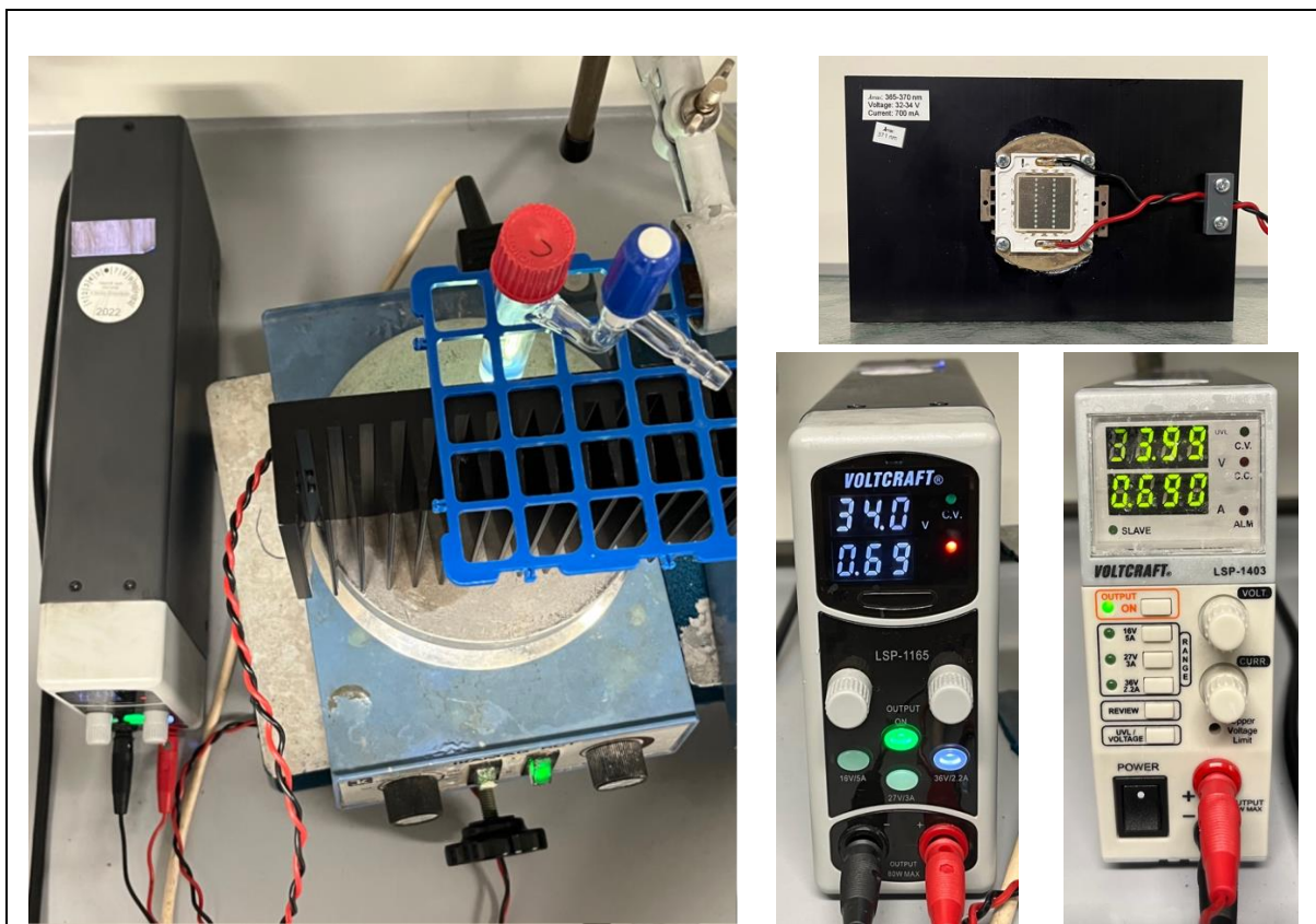
Figure S1: Photoreaction set-up (left). LED chip construction, powered by either a Voltcraft LSP-1165 or an LSP-1403 power supply (right).
