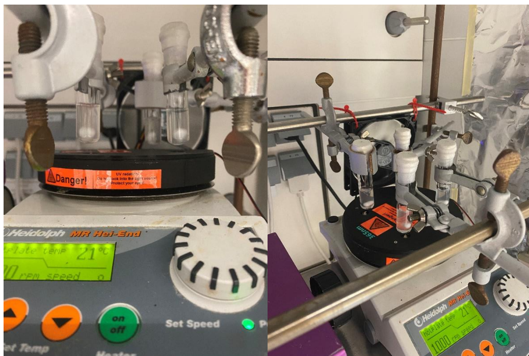
Figure S2. Reaction set up for photocatalyzed energy transfer reaction. (Left: side view, right: diagonal view)
