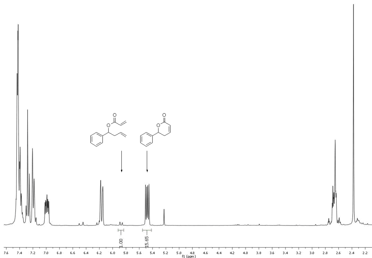
Figure S2: A typical ^1\text{H} NMR spectrum of a crude reaction mixture for RCM of acrylate 3a .
