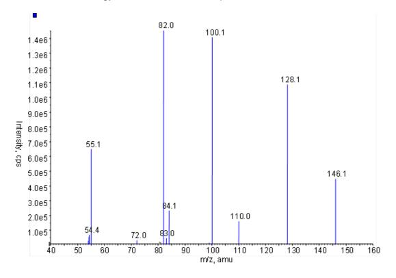
Tandem mass spectrometry: MS<sup>2</sup> of molecule peak 146 [M + 1]<sup>+</sup>
