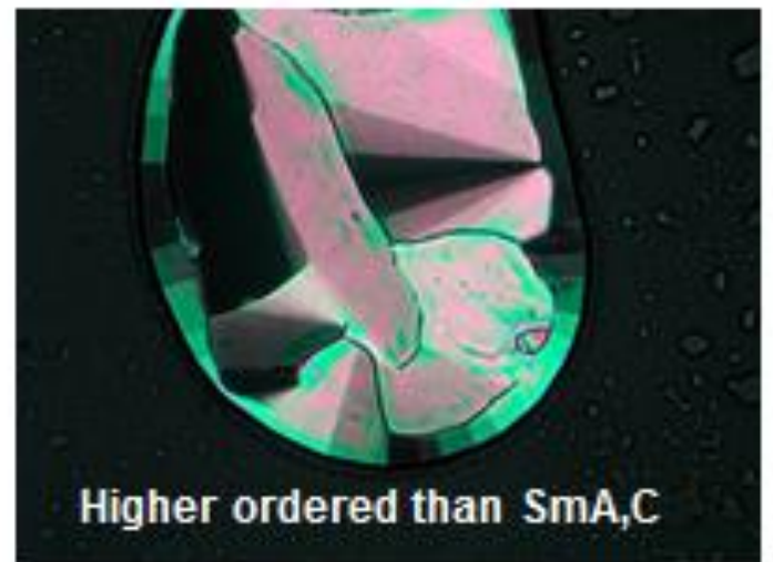
Textures of 8b under crossed polarizers upon cooling from the isotropic liquid (magnification 200 \times , cooling rate 5 K/min)
