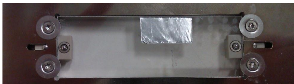
Figure S4: Photo of the aluminium rectangle backing. The aluminium rectangle is not in contact with the metal frame.
