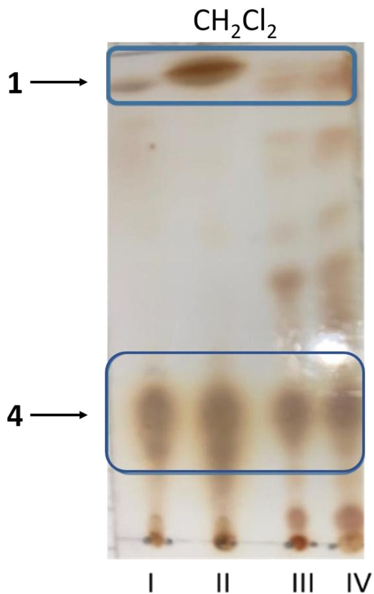
**S1.** Chromatographic profile of amination reactions of **1** with different molar ratios of CAN to produce **4**. 1:1 (reaction I), 1:2 (reaction II), 2:5 (reaction III), and 1:3 (reaction IV).
