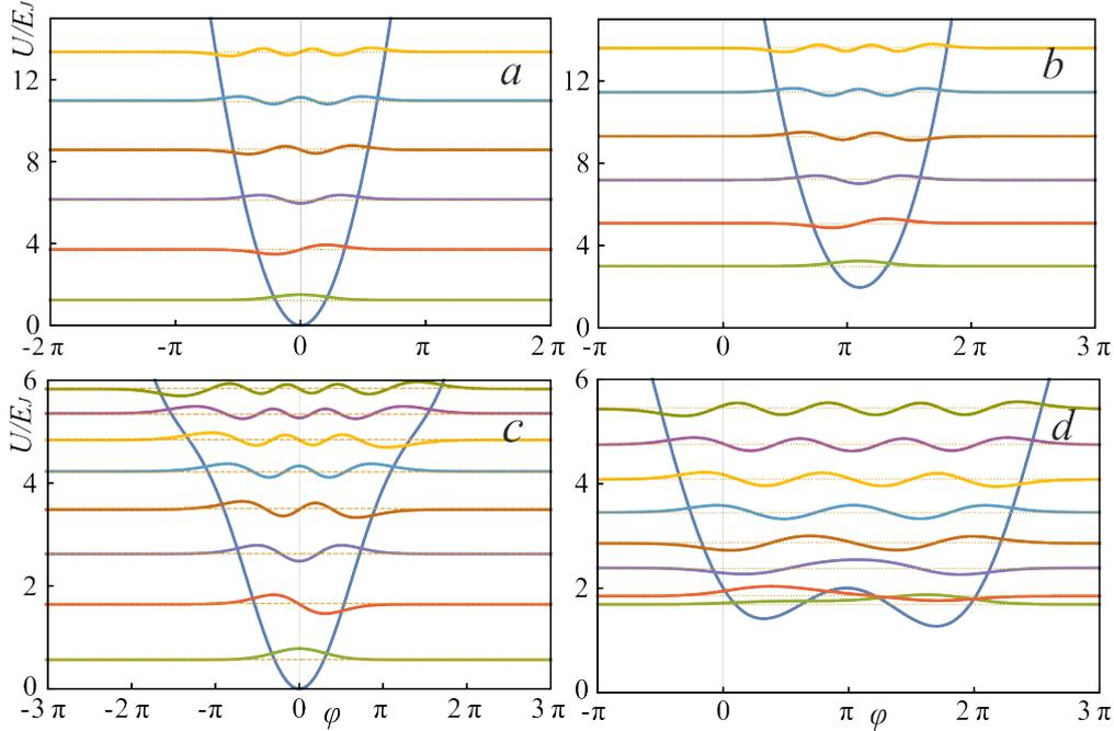
**Figure 2:** The energy spectrum and adiabatic (instantaneous) wave functions are represented at the initial time  $t = 0$  (a, c) and at the rise of the applied flux,  $t_1 = 500$  (b, d) for the inductance value  $l = 0.1$  (a,b) and  $l = 2.5$  (c, d). The parameters of the system and the input magnetic flux are:  $E_C = 0.5E_J$ ,  $l_a = l + 1$ ,  $l_{out} = 0.1$ ,  $D = 0.008$ ,  $A = 4\pi$ ,  $t_2 = 3t_1$ .
