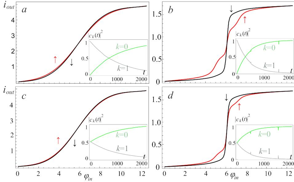
**Figure 10:** The neuron activation function for  $l = 0.1$  (a, c) and  $l = 2.5$  (b, d) when the cell is initialized in the first excited level (a, b) and in the superposition of two basic states (c, d). The input flux parameters are as follows:  $D = 0.008$ ,  $A = 4\pi$ ,  $t_1 = 500$ ,  $t_2 = 3t_1$ ; the renormalized coupling constant  $\lambda = 0.005$ . The insets present the corresponding populations  $|c_k(t)|^2$  of the energy levels.
