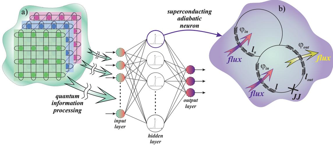
**Figure 1:** (a) Sketch of a flexible hybrid system consisting of a classical ANN having configuration (synaptic weights) dynamically adjusted by a quantum co-processor. (b) Schematic representation of the  $S_Q$ -neuron providing nonlinear magnetic flux transformation.
