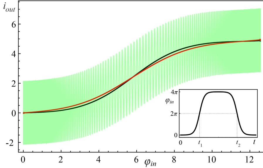
**Figure 3:** The neuron activation functions for  $l = 0.1$  and different initial states: the black curve corresponds to the ground initial state  $\psi_0(\varphi, 0)$ , the red one — to the first excited state  $\psi_1(\varphi, 0)$ , and green curve corresponds to the superposition of states  $(\psi_0(\varphi, 0) + \psi_1(\varphi, 0))/\sqrt{2}$ . Parameters of the input magnetic flux are  $D = 0.008$ ,  $A = 4\pi$ ,  $t_1 = 500$ ,  $t_2 = 3t_1$ .
