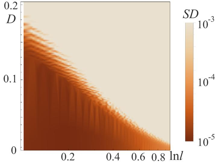
**Figure 9:** The value of the square of the standard deviation,  $SD$ , of the  $S_Q$ -neuron activation function from the mathematical sigmoid (16) for various inductance  $l$  values and rise/fall rates,  $D$ , of the input flux  $\varphi_{in}(t)$ . At the initial moment, the system was initialized in the ground state. The parameters of the system and the input flux are as follows:  $A = 4\pi$ ,  $l_a = l + 1$ ,  $l_{out} = 0.1$ .
