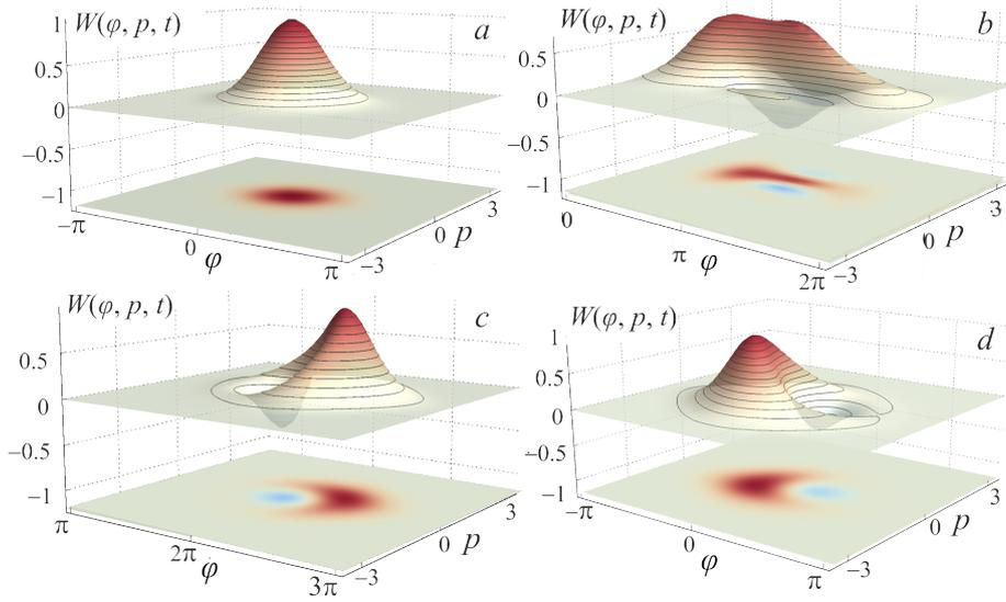
**Figure 7:** The evolution of the Wigner function of the  $S_Q$ -neuron with  $l = 2.5$  initialized in the ground state under the action of the input flux  $\varphi_{in}$  at the moments  $t = 0$  (absence of  $\varphi_{in}$ ) (a);  $t = 500$  (the middle of the increase of  $\varphi_{in}$ ) (b);  $t = 1000$  (the plateau of  $\varphi_{in}$ ) (c);  $t = 2000$  (absence of  $\varphi_{in}$ ) (d). The input flux parameters are equal to those shown in the figure 6.
