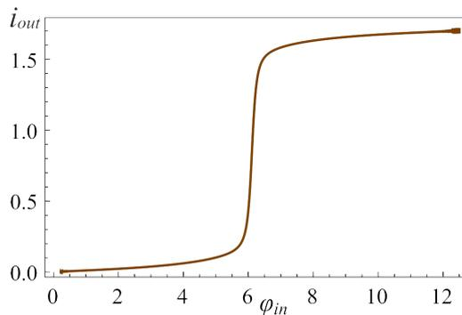
**Figure 8:** The activation function of the neuron with  $l = 2.5$  initialised at  $t = 0$  in the ground state. Here the parameters are  $D = 0.0002$ ,  $A = 4\pi$ ,  $t_1 = 10000$ ,  $t_2 = 3t_1$ .
