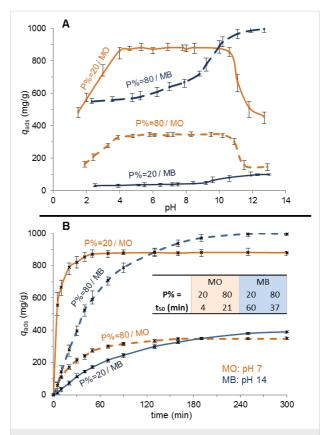
**Figure 2:** A) pH Values at which NP-PEIP20 and NP-PEIP80 adsorb a maximum amount of dye. MO is better adsorbed in the range of pH from 4 to 10. P% does not impact the pH range but the amount of removed dye. For MB, the higher the P% is, the better the extractions are, regardless of the pH value. Maximum amounts are removed at basic pHs. B) Adsorption of MO is faster than that of MB, regardless of the percentage of phosphonate groups.
