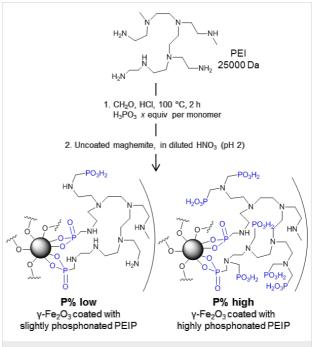
**Figure 1:** Synthesis of NP-PEIP. The number of phosphonates depends on the number of equivalents of phosphorous acid used.
