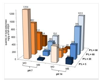
**Figure 4:** Removed amounts of MO and MB dyes by NP-PEIPx at pH 7 and 14. P% significantly affects adsorption of MB and MO. At neutral pH, much more MO is eliminated than MB, while the contrary is observed at basic pH.
