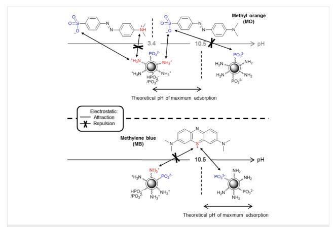
Figure 3: Prediction of the best range of pH values for electrostatic attractions between NP-PEIP and MO and MB dyes. Only the major interaction (i.e., ammonium) is represented. For MO, an interaction occurs with sulphates and ammonium groups, until the  $pK_a$  (NH<sub>3</sub>+/NH<sub>2</sub>) is reached. Cationic MB is attracted by the phosphonate groups introduced on PEI at basic pH values.
