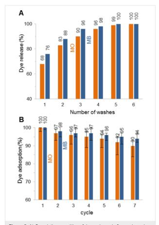
**Figure 5:** A) Cumulative quantities of dyes released after each wash. MO is desorbed from NP-PEIP05 with sodium hydroxide aqueous solution, MB from NP-PEIP90 with diluted nitric acid. B) The efficiency of the dyes extraction remains high after several adsorption/desorption cycles.
