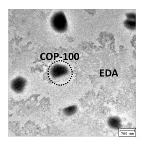
Figure S1: TEM image of COP-100 treated with EDA at 100 °C.
