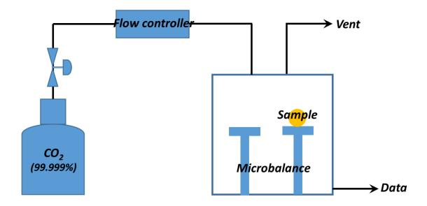
**Figure S3:** Schematic illustration of the experimental set-up for a gravimetric uptake of CO<sub>2</sub> using thermogravimetric analysis instrument.
