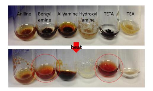
**Figure S2:** Variation of liquid amines for dissolving COP-100 at 100 °C. TETA: triethylenetetramine, TEA: triethylamine.
