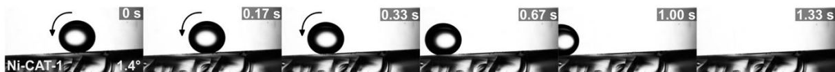
Figure S5.6 An image series of a self-cleaning surface experiment (3 fps) with DCM as an oil droplet placed on a tilted nanostructured Ni-CAT-1 film (tilt angle of 1.4°).
