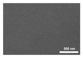
Figure S1: SEM image of a continuous silver layer deposited using 4000 laser pulses at room temperature.
