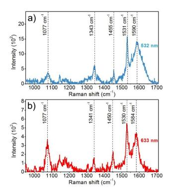
Figure S2: Raman spectra of the pMA monolayer formed on the platinum foil, recorded using two excitation wavelengths: a) 532 nm, b) 633 nm.
