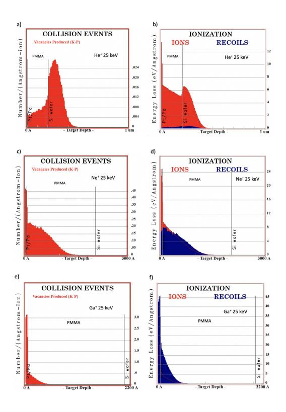
**Figure S1:** SRIM simulations of collision and ionization in the 5 nm  $Pt_{60}Pd_{40}/200$  nm PMMA samples, irradiated with (a, b) He<sup>+</sup>, (c, d) Ne<sup>+</sup>, and (e, f) Ga<sup>+</sup> FIBs.
