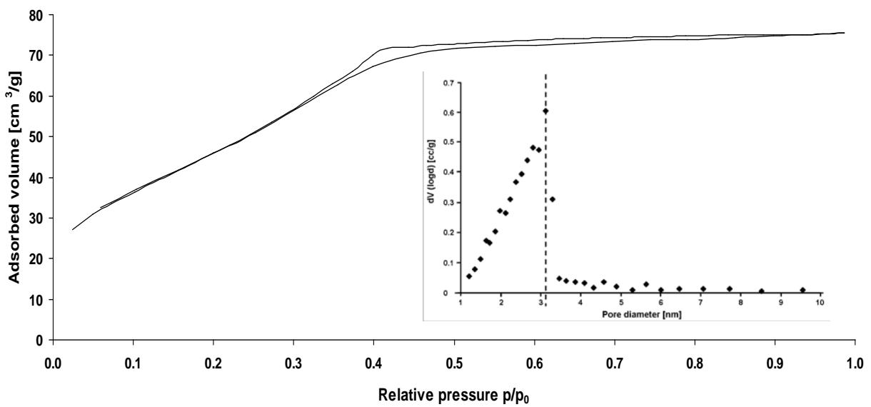
**Figure S1:** Nitrogen sorption measurement of porous titania. The inset shows the pore size distribution evaluated by the BJH method from the desorption branch of the isotherm.
