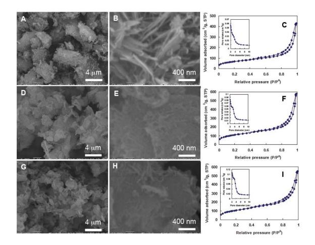
**Figure S5**: SEM images (A, B, E, F, H and I) and BET results (C, G and J) of nanostructured silicas synthesized by using bases of  $Et_4NOH$  ([OH]/[EI] = 1.6) (A–C), LiOH ([OH]/[EI] = 2.7) (D–F) and KOH ([OH]/[EI] = 3.2) (H–J). 0.5 g of LPEI-HCl was dissolved into 6 mL of water for LPEI self-assembly induced with various bases. The silica deposition was performed by stirring a mixture of 1.5 mL of MS51 and 15 mL of aqueous dispersion of LPEI aggregates for 4 h at room temperature.
