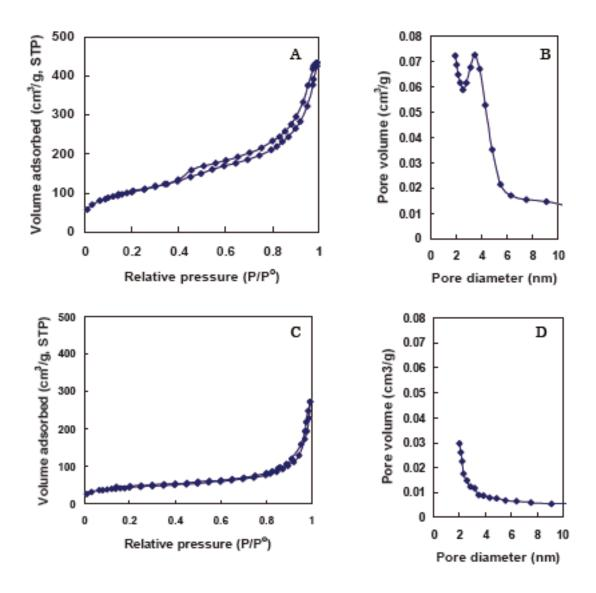
**Figure S2**: N<sub>2</sub> adsorption/desorption isotherms (A and C) and BJH pore-size distribution curve obtained from the adsorption branch (B and D) of silica nanotube (A and B) and silica nanoribbon (C and D). The synthesis conditions are the same as those of the samples shown in Figure 4. The sample was calcined at 800°C in air for 3h with at heating rate of  $2.5^{\circ}$ C per min.
