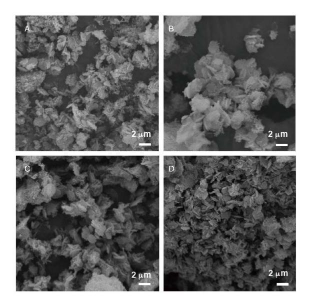
**Figure S3**: SEM images of silica nanostructure synthesized by using MS51 concentrations of 23.1 % (A), 9.1 % (B), 4.6 % (C) and 1.1 % (D). Other synthetic conditions are the same as those used in Figure 6.
