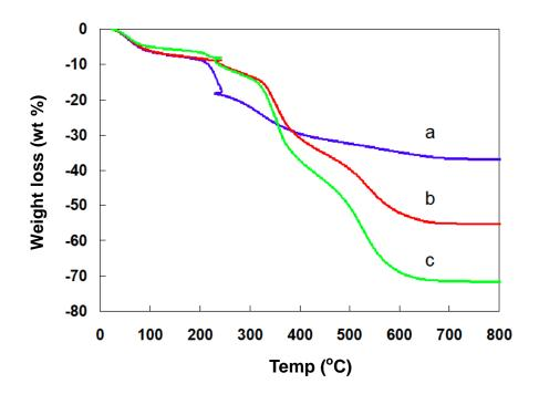
**Figure S6**: TGA curves of LPEI@silica hybrid nanotubes (a), and the nanotubes adsorbed with one layer of PSS (b) and two layers of PSS (c).
