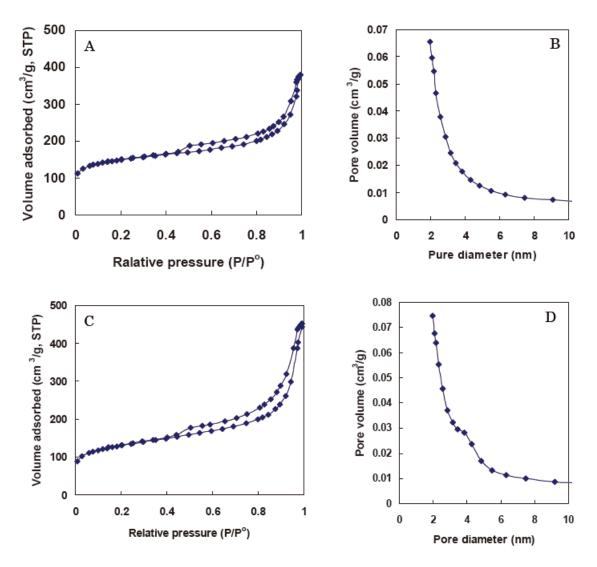
**Figure S4**: N<sub>2</sub> adsorption/desorption isotherms (A and C) and BJH pore-size distribution curve obtained from the adsorption branch (B and D) of nanostructured silicas synthesized under the feeding ratios of [OH]/[EI] of 0.8 (A and B) and 3.2 (C and D). The synthesis conditions are the same as those of the samples shown in Figure 7. The sample was calcined at 800°C in air for 3h with at heating rate of 2.5°C per min.
