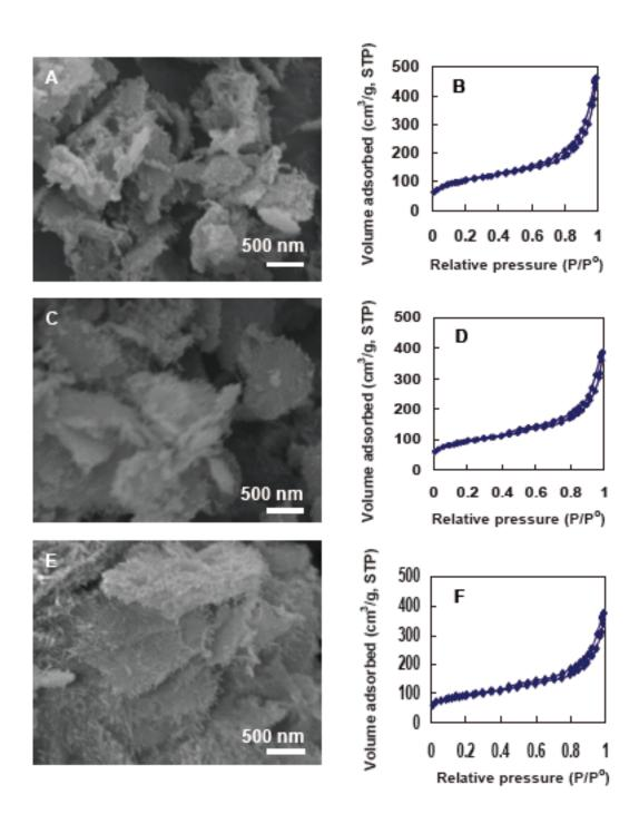
**Figure S1**: SEM images (A, C and E) and  $N_2$  adsorption/desorption isotherms (B, D and F) of silica nanotubes synthesized with silicification times of 5 min (A and B), 60 min (C and D) and 240 min (E and F). The synthetic conditions for LPEI aggregates and silica deposition are the same as those used for Figure 3.
