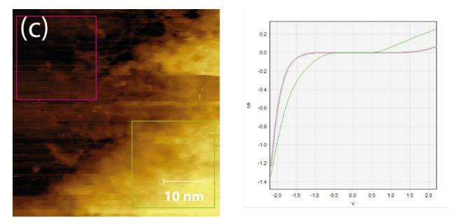
**Figure S2:** (a) silicon clusters on top of  $MoS_2$  after deposition of 1.4 monolayers of silicon. The purple and green boxes indicate the locations where a grid scan is performed. Each grid did consist of 100 curves. (b) The average of the recorded I(V) curves on top of the cluster (green) is significantly different from the average of the curves recorded on  $MoS_2$  (purple).
