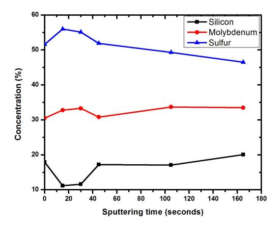
Figure S3: Atomic concentration of Si, Mo and S as a function of the sputtering time. The sputter current used is  $0.33 \,\mu\text{A}$  with an estimated spot diameter of 2 mm.
