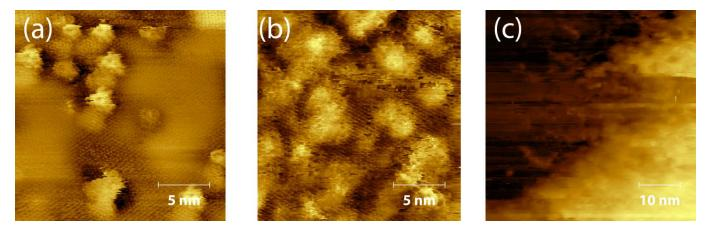
**Figure S1:** Topography of the MoS<sub>2</sub> surface as a function of the amount of deposited silicon. (a) 0.2 monolayers. Here transitions between hills and valleys are visible. The recurring feature is a tip image. (b) 0.8 monolayers. The sample becomes rougher and more difficult to image. (c) 1.4 monolayers. Silicon clusters are visible on top of the MoS<sub>2</sub>.
