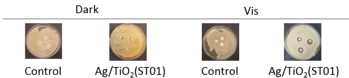
Figure S5: Antifungal activity of silver-modified photocatalysts against C. albicans after 48 h in the dark condition and under visible light.
